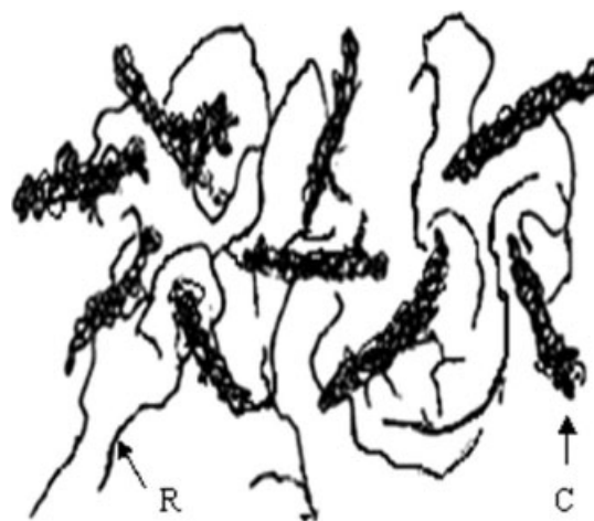
Figure 13 Clay chain network in composite (R is rubber chain and C is clay).
